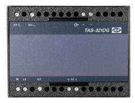
Powerful, fast and compact, the units in DEIF's transducer range measure sinusoidal alternating voltage and/or current signal and provide output signal as direct current or voltage signal proportional to measurements for PLCs, PCs, microprocessor control, indicators, alarm units etc.
