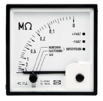
DEIF's SIM insulation monitors supervise the insulation resistance between an insulated voltage distribution network and an earth/safety cable. The advanced measuring sequence performs an automatic offset adjustment to eliminate possible effects of uneven stray capacitance and DC voltages.
