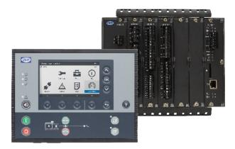
The PPU 300 Paralleling and Protection Unit is a highly configurable controller designed for marine use. The controller contains the functions required to protect and control a generator and its breaker (specifically, a diesel generator, a shaft generator, a shore connection, or a bus tie breaker). You can connect up to 12 controllers to create one system, with load sharing sections.
