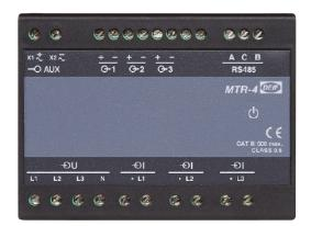
Efficient, fast and flexible, the programmable MTR-4 transducer offers the same performance as up to four standard transducers, measuring and calculating AC voltage, AC current, active/reactive apparent power, power factor, frequency, kWh, kvar, THD, dynamic and maximum demands.
