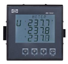
DEIF's multi-instruments for measurements and monitoring of single-phase or 3-phase electric energy distribution networks cover readings of more than 50 parameters.
