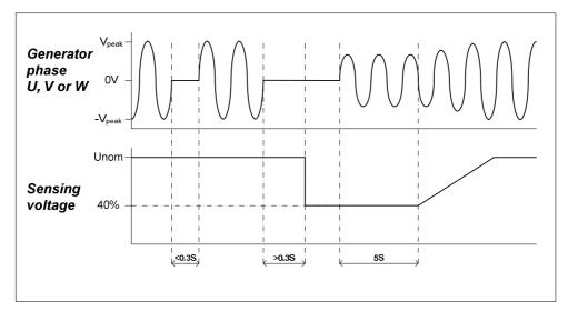
The phaseloss protection validates the presence of all three generator phases on the sensing terminals U, V and W. When one of the three phases is not sensed anymore for more than 300ms the AVR decreases the generator voltage setpoint to +/- 40% of Unom. If the error condition is relieved for 5s, the generator voltage is ramped up again to nominal voltage.
