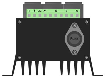
To prevent consequential damage in case of an AVR or generator failure, the AVR supply is fused by a 20A ultra rapid fuse.
